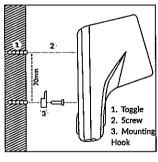
WALL MOUNTING -NOT HARD WIRED Drill 2x 6mm diameter holes, separated vertically at a distance of 70mm. Place toggles (supplied) in the holes. Use 1x screw to secure the small mounting hook to the wall. Slide the wall unit on to the mounting hook. Push the second screw through the hole in the wall unit and screw the unit to the wall. Place cover plate over the access hole at the bottom of the front wall unit panel.
